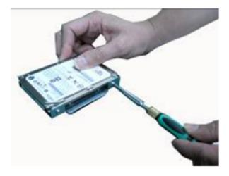
Step 6 Install and fix the HDD through the bottom, next, plug the power cable in HDD.
